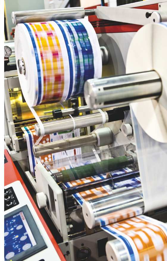
The Xeikon 3300's reworked technology yields 1,200-dpi print resolution.
